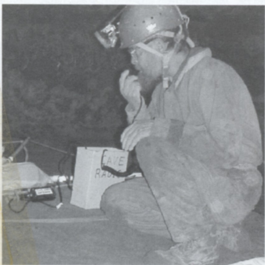
Donald G. Davis with the 185 KHz induction radio for a scheduled call to the surface.
